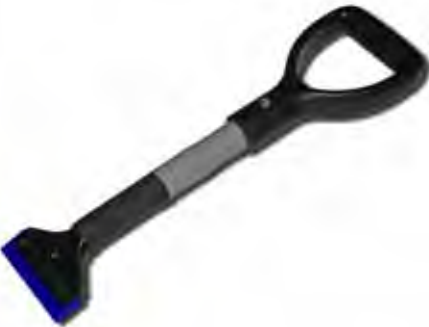
THOR'S HAMMER The Thor's Hammer is strongly recommended when installation of 6 mil and greater security window film is being installed. This tool allows for the window film installer to gain extra leverage with a stiffer squeegee blade which assists in the removal of mounting solution with thicker window films. Removal of the maximum amount of mounting solution will assist in decreased drying times.
