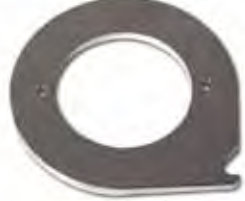
F FS942 1/4" THICK SHIM FOR 3" FILM HAN- DLER ROLLER ASSEMBLIES (1 SHIM) This shim is designed to eliminate side to side film movement during the slitting process. This shim is 1/4" thick and designed to be used with a 3" Roller Assembly on the Film handler window film cutting machine.
