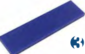
5" BLUE MAX SQUARED NARROW SQUEEGEE BLADE When dealing with safety window films of 6 mil or greater, it is imperative that the squeegee blade has very little flex to facilitate adequate mounting solution removal. The narrow design allows less squeegee blade to protrude from the handle which serves to stiffen the blade. This Blue Max blade was designed specifically for these safety film applications and should be considered a must for any substantial security window film work. (This blade is specifically designed for use in HS1006 handle)
