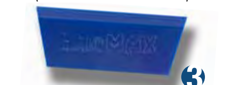
8" BLUE MAX BLADE WITH BEVEL Now available in the larger 8" size, the Blue Max is the original beveled squeegee and still considered by many in the window tinting industry to be the best blade available. The Blue Max is harder than the Orange Crush or the Clear Max making it terrific at removing mounting solution from high performance and ceramic window films. (Use with HS1046 handle)
