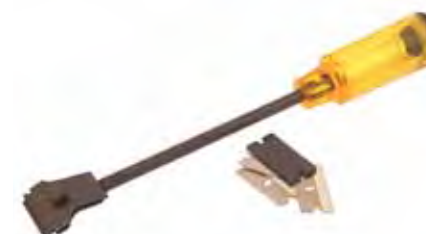
SR109S 1" HANDLED CLIP SCRAPER WITH THUMB SCREW Very similar to a standard handled clip scraper. However, this tool comes with a thumb screw to hold the blade tighter if more scraping force is required. (Uses any standard 1" single edge razor blade)
