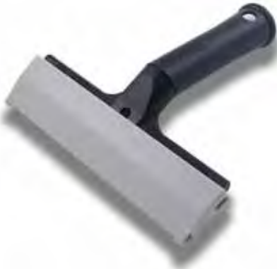
SR107A 6" TRIUMPH ANGLED SCRAPER This is essentially the standard Triumph 6" Scraper with a 30 degree angled head for better ergonomics and to apply more leverage. (Uses Triumph blades SR108 & SR108SS)
